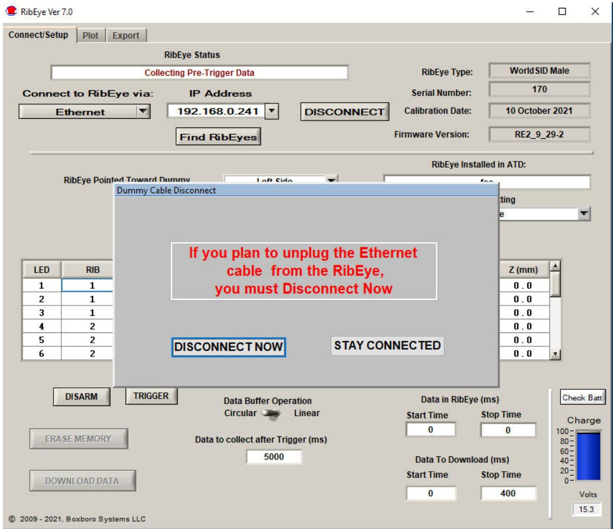
If you *do* plan to disconnect the cable, you must click on the “Disconnect Now” button. This will close communications to the RibEye so that disconnecting the cable will not lock up communications. If you *do not* plan to disconnect the Ethernet cable, you can click the “Stay Connected” button. After the test is completed and the Ethernet cable is plugged back in to the Trunk Box, you can click on the “Connect” button to re-establish communications with the RibEye.
