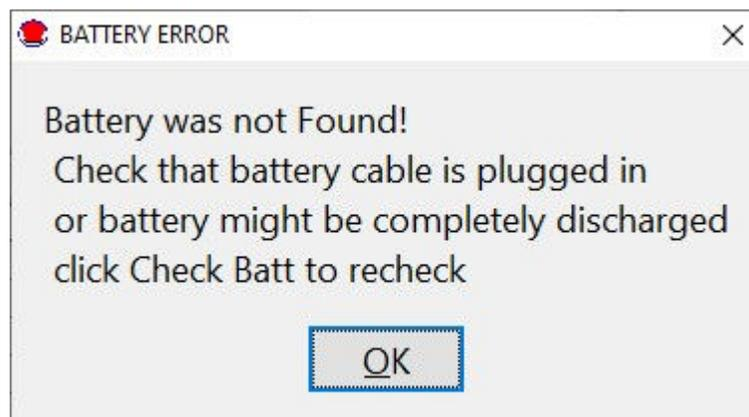
When you arm the RibEye, it will display a different error message (Figure 17) if the battery is less than 50% charged. When a test is complete, the RibEye will read the battery fuel gauge again and display the charge level on the screen.
