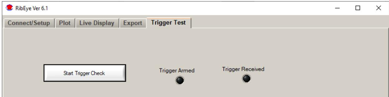
If you click on the “Start Trigger Check” button, the RibEye will arm the trigger circuit and the “Trigger Armed” light will light up as shown in Figure 34.
