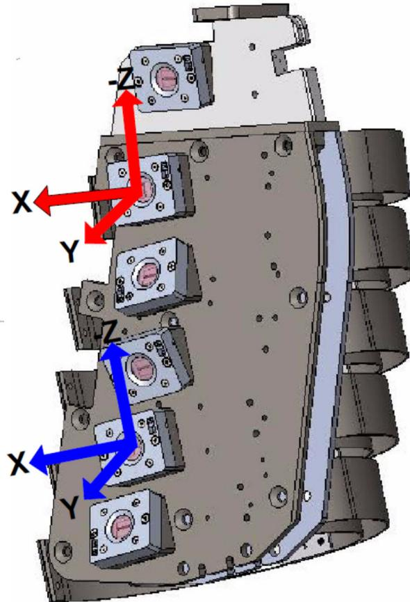
The Length Change for a LED at time  $t$  is the initial vector length from the LED to the RibEye origin in the XY plane minus the vector length from the LED to the RibEye origin at time  $t$ .
