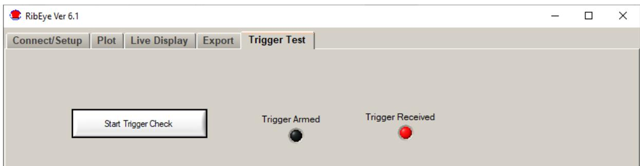
Remember that the trigger setting on the main screen controls whether the RibEye is looking for a rising-edge or falling-edge trigger. The trigger setting operation is described in Section 2.5.
