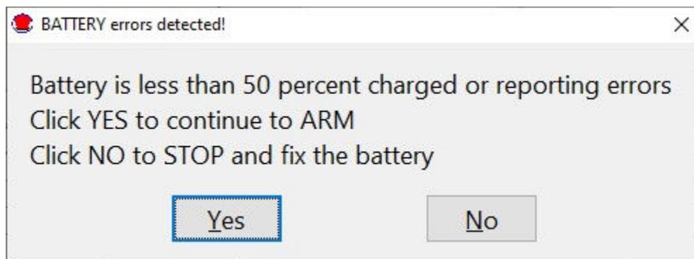
If the battery has been completely discharged, the fuel gauge chip will be reset, and it will not know the charge level. Then you will get the error message shown in Figure 18. To fix this, you must fully charge the battery (until the charger light is solid green) and then click on the “Fully Charged” button. If you close the screen shown below, it will come back again when re-connecting to the RibEye or clicking on the “Check Batt” button.
