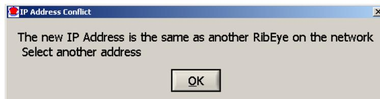
In rare circumstances, another device on your network uses the same protocol to change its IP address as the RibEye does. If this occurs, you will get the error message shown below. To prevent changing the address on the other device that uses the same protocol, you should remove the RibEye from your network and connect the RibEye directly to a PC and change its address. Then you can put the RibEye back on the network.
